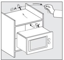
Slide the appliance into the housing unit, and pull the cable with the plug\* through the back of the unit.
